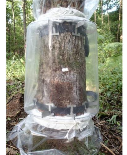
Cylindrical chamber for CH<sub>4</sub> flux measurement
